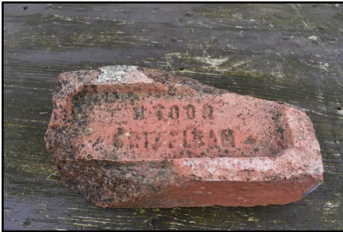
Machine made pressed bricks made when Henry Toon was operating the brick works on the Lower brand
