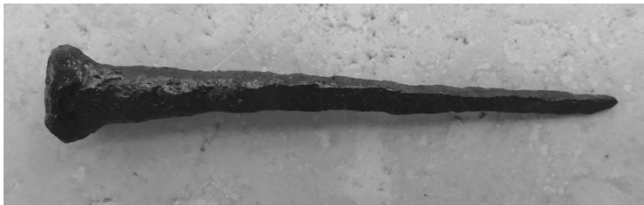
An example of a rusted handmade nail, of the type that would probably have been made by Charlie Marson
