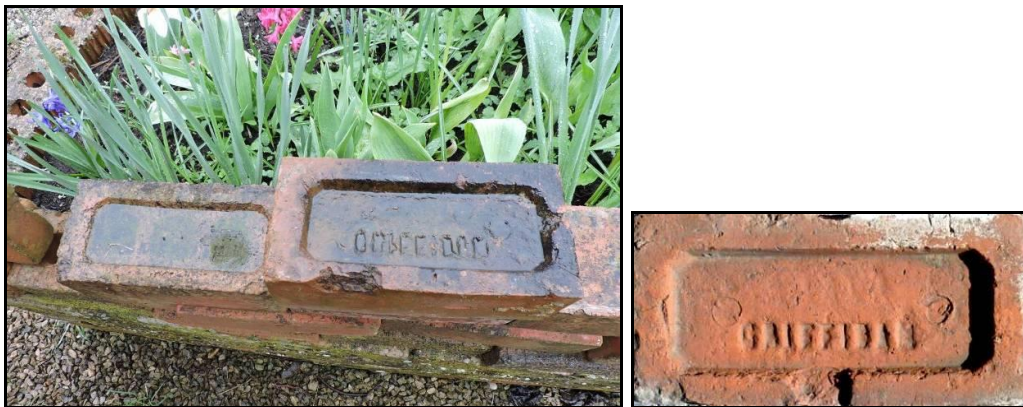
The above photographs are examples of pressed bricks which have “Griffydam” impressed into them, suggesting they were made between 1877 and 1880 when that part of the Lower Brand came into Griffydam.
