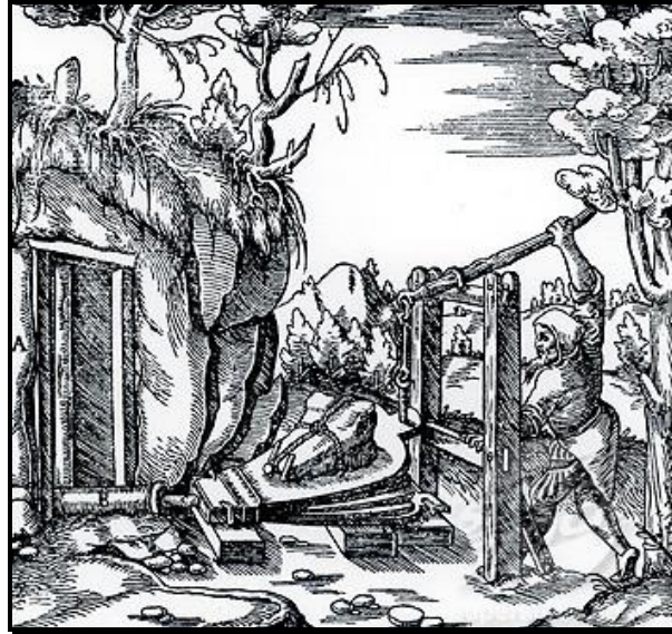
Ventilating a mine using bellows
