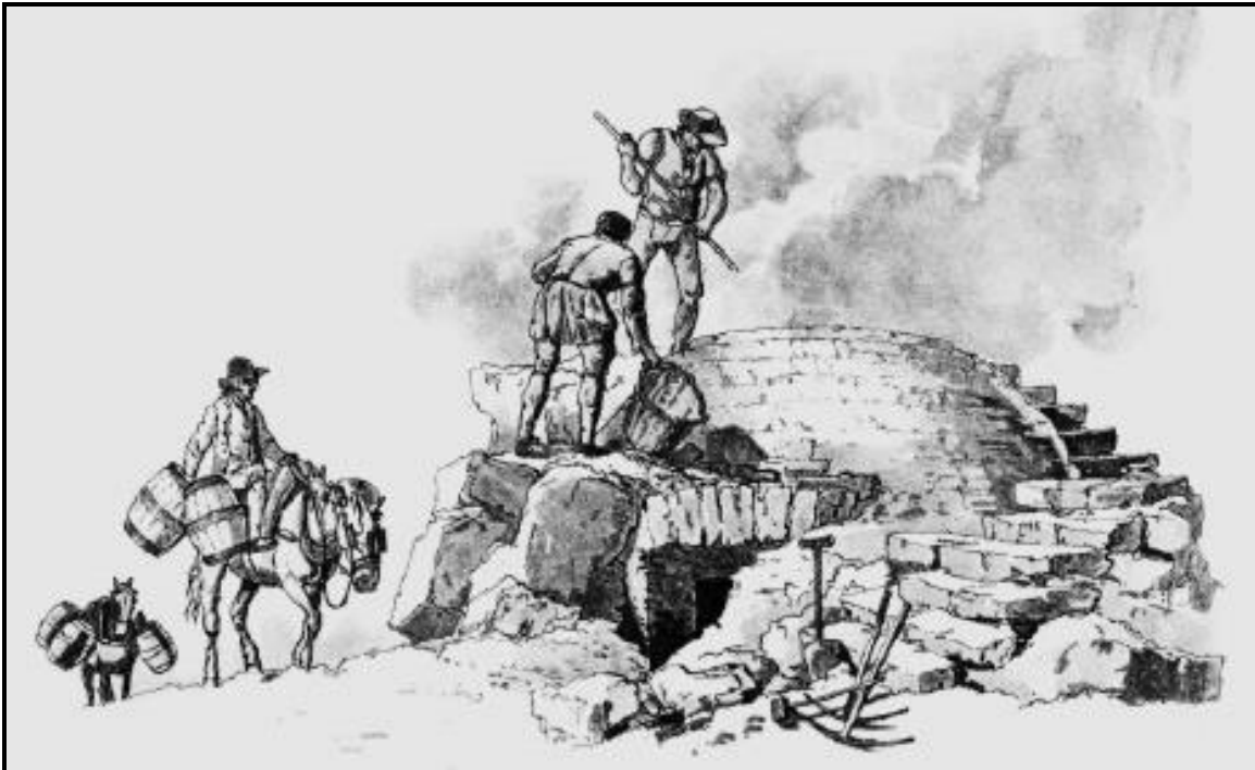
An etching by W. H. Pyne 1806 of a field lime kiln with fuel (slack coal) being transported to it by Packhorse
