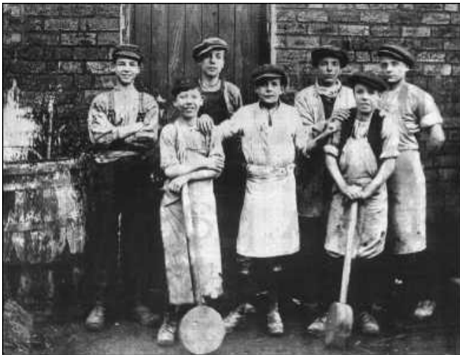
Pottery lads in 1921 with two mawls, the tool used for bottom knocking.
