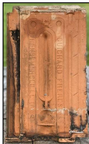
Example of a sophisticated old design of interlocking roof tile by Guichard Freres St Henri, Marseille, France
