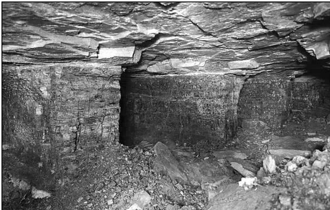
Photograph of “Stall and Pillar” type working
