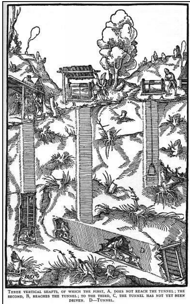
Timber lined shaft mining
