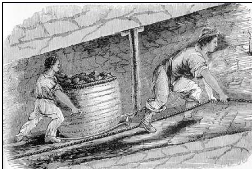
Illustration of coal being pulled along in Corves (hazel twig baskets) on sleds or sledges by a woman and child
