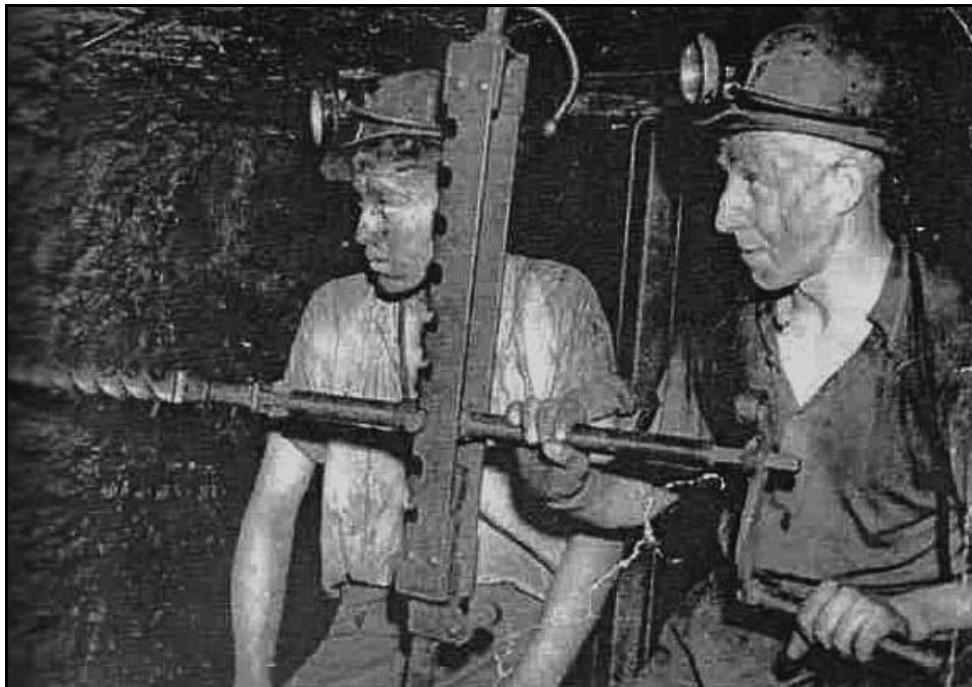
“Mighty” Jim (Jack) Wardle with his son Willie, “manually” drilling holes in the coal face for explosives
