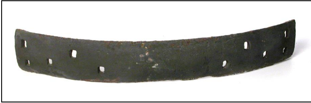
A strake made from Wrought Iron - 120mm wide by 715mm long
