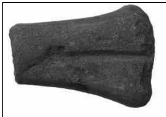
A typical piece of whetstone from the quarry prior to dressing
